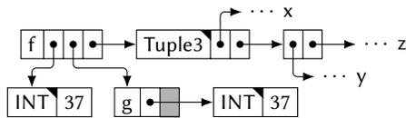
Figure 1: The runtime memory layout of a Clean program.
